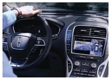
Onboard cameras present the driver with an available 360-degree view of the vehicle's surroundings. This is a Nautilus interior image.
