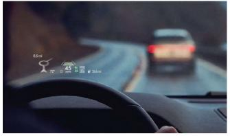
Highly useful vehicle system and driving info is shown right in front of the driver, on the windshield in the available head-up display.<sup>2</sup>
